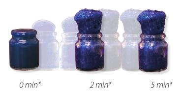
2 min\*: Foaming action complete; 5 min\*: Material completely cured. Total Expansion 160%
