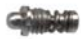
PRECI-52 INTERNAL MALE # 1563 male U insert 2 pcs ø ball: 1.55 mm - length: 5.8 mm - total ø: 2.6 mm
